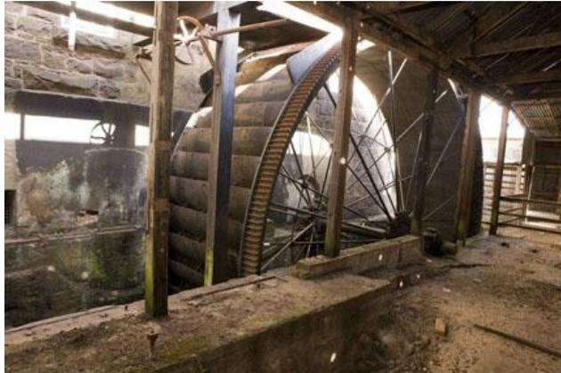
**Figure 86.** Waterwheel at the Anderson's Flour Mill, Smeaton, Victoria (1861) (source:VHR 1521)
