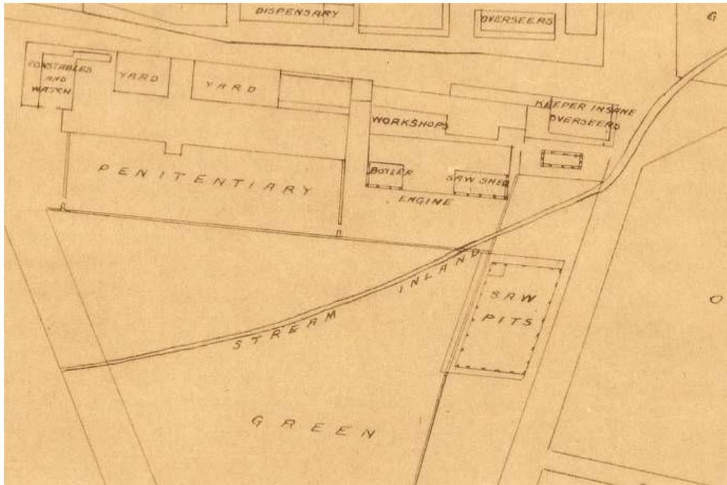
**Figure 33.** Site plan of the Penitentiary and new workshop complex, late 1850s. Note the surviving overseer’s quarters at the west end of the site. Covered saw pits were built on the north side of Settlement Creek (which had been covered over). (Archives Office of Tasmania, ref. PWD266-1-1775)
