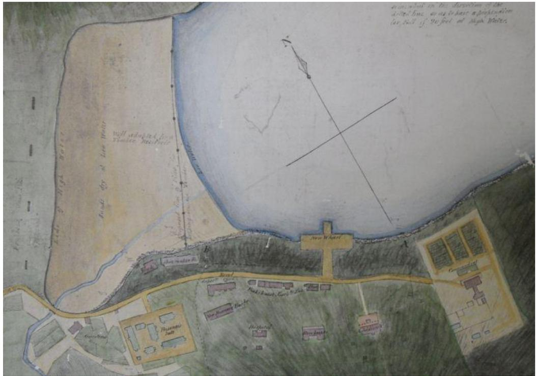
**Figure 2.** Detail from J.W. Hughes 1833, 'The Settlement of Port Arthur' showing the Shoemakers' and Blacksmiths' Shops erected in 1831 on the south side of the cove. Note that they are located on the edge of a sandy area submerged at high tide, which was later reclaimed. (PAHSMA ref. HM 1833/1)
